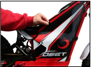
(1.) Release Velcro straps
