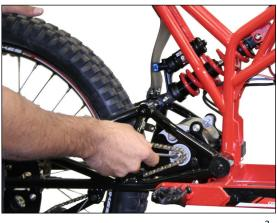
Next, push down on the spring loaded chain tensioner, which will relax the chain slightly. Whilst doing this, you can lever the front sprocket loose on the shaft with the screwdriver, pulling the sprocket in the direction shown in *image 5*.
